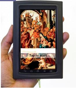
The new TourMedia Touch features an Android operating system and a large 5" touch screen with a 480 by 800 resolution. Additionally, the device supports multi-platform social media integration. The TourMedia Touch player is WIFI enabled. Proprietary software distributes software updates and content in parallel to a network of connected modular racks and players.
